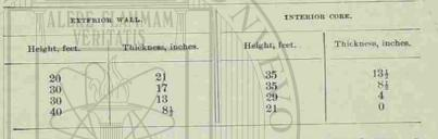
Exterior diameter at base is 15 feet 6 inches; batter,  $r_8^{-1}$  inches from the bottom to 8 feet from the top, then straight. Space between walls, 16 inches at bottom, diminishing to nothing at the top of core wall.
