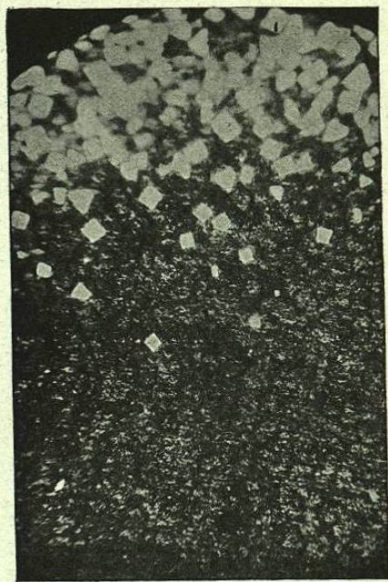
Fig. 16. Alloy of 90 per cent Tin, 10 per cent Antimony. Showing how the Cubes of Tin Antimonide (Sn Sb) have risen by Gravity to the Top of the Ingot. Vertical Section of the Ingot. Prepared by William Campbell in the Author's Laboratory.
