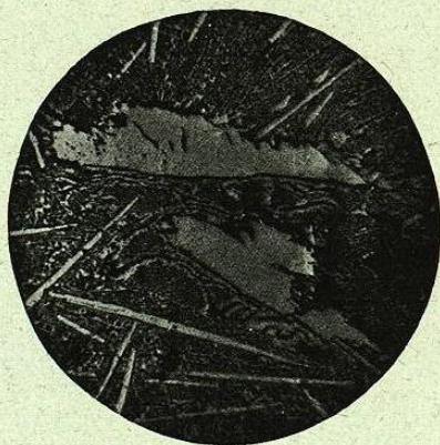
Fig. 40. Cast Iron Showing Plates of Cementite and Eutectic. Section parallel to cooling surface.
