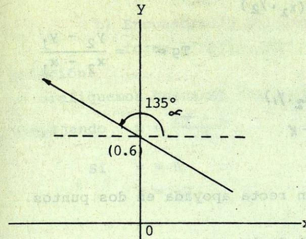
$$\begin{aligned} \tan 135^\circ &= -1 \\ m &= \tan \alpha \\ m &= -1 \\ \therefore b &= 6 \\ \underline{\text{ec. } y} &= \underline{-x + 6} \end{aligned}$$
