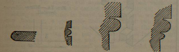
Fig. 41. Rounded Edge. Fig. 42. Bead. Fig. 43. Torus. Fig. 44. Torus and Bead.
