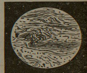
FIG. 2.—Microscopic Structure of Obsidian.—A volcanic glass, with numerous microlites, which have been drawn out in a general direction during the flow of the melted rock (fluid-structure). (X 18 diameter.)
