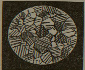
FIG. 5.—Microscopic Structure of Saccharoid white Marble (Carrara).
