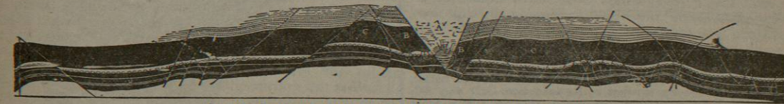
FIG. 49.—Section of a faulted part of the thick coal of South Staffordshire.
