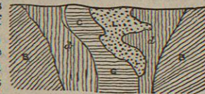
Fig. 6.—Vertical Section, Altenberg. B, slate; d, dolomite; C, calamine; L, clay.
