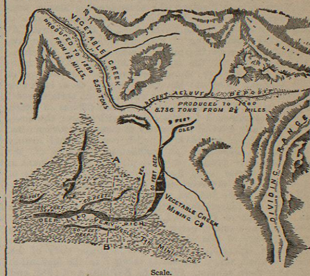
FIG. 105.—Sketch Map of Part of Vegetable Creek, New South Wales, showing recent and ancient tin deposits. The stippled part represents tin-bearing alluvium. The shaded part AB denotes basalt which has covered the lower portions of the ancient tin-bearing alluvia (deep leads), as explained in fig. 106. The rest is granite.
