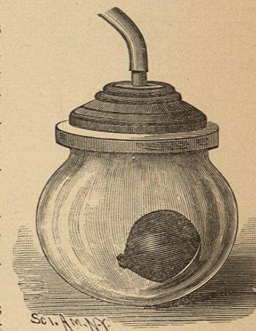
Dilatation of Balloon in a Vacuum.
