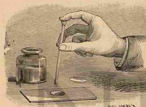
Transferring Objects to the Slide.
