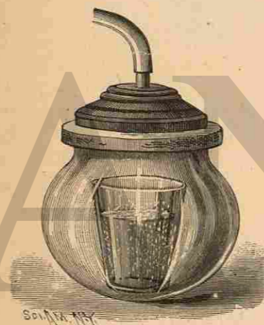
Water Boiling in Vacuo.
