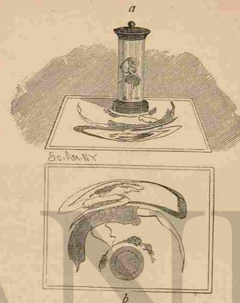
a, Convex Cylindrical Mirror. b, Distorted Picture to be viewed in Mirror
