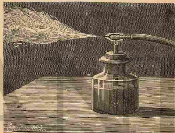
Atomizing Petroleum Burner.
