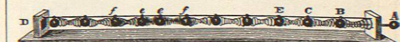
FIG. 384.—Illustrating Passage of an Air Wave. The balls, E, C, B, etc., represent air particles and the springs the elastic force restoring them to position. (After Tyndall on "Sound.")
