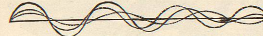
Fig. 392.—The Two Broken Lines Represent Air Waves of Slightly Different Vibration Rates. The solid line represents the "beats" or variations in sound intensity produced by the algebraic addition of the first two.
