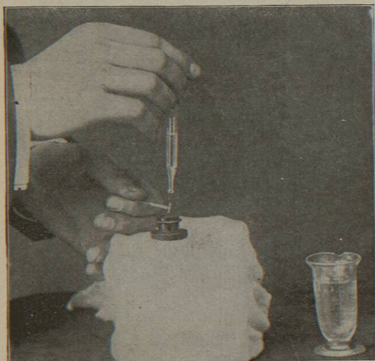
FIG. 579.—Von Fleischl's Hæmoglobinometer. Washing drop of blood from capillary tube with water into one side of double well.
