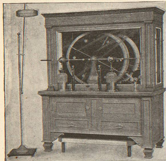
FIG. 1835.—Wagner Static Machine, with Four Revolving Mica Plates (diam. 28 in.) and Four Stationary Glass Plates (diam. 31 in.).
