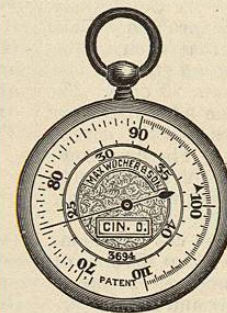
FIG. 4701.—Immiscible's Avitreous Thermometer. (Exact size.)
