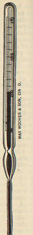
FIG. 4700.—The Minute Thermometer. The column of mercury appears magnified by means of the so-called lens front.
