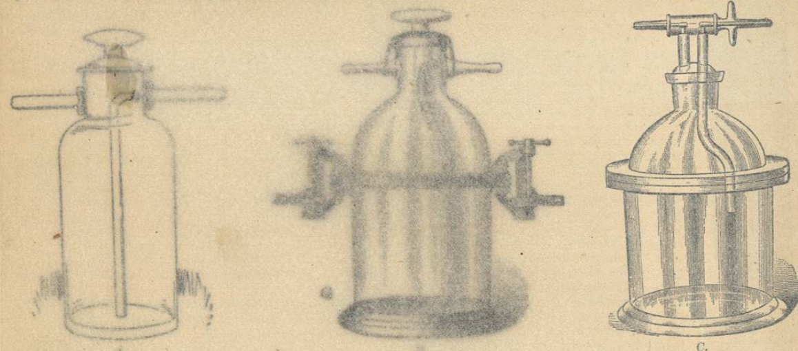
FIG. 5094.—Novy's apparatus for anaerobes. A, Bottle for tube cultures; B, Jar for plates; C, Jar for plates with special stopcock for vacuum cultures.
