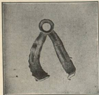
FIG. 2386.—Ruptured Mauser Mantle, to illustrate the Tendency to Complete Longitudinal Fissuring. (Makin.)
