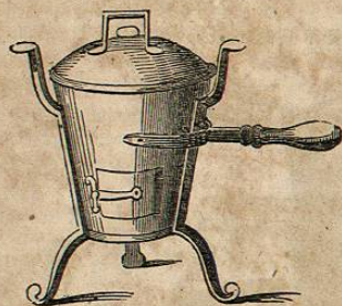
Closed Furnace and Cover.
