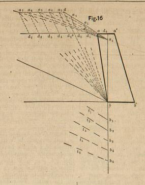
triangles bda, bda, bda, bda, etc. pro- other form than that above treated, the portional in area to the lines ea, ea, etc. vertical plane against which the pressure Hence the weights of the prisms of earth is determined should still pass through baa, baa, etc., are proportional to ad, the lower back edge of the wall.
