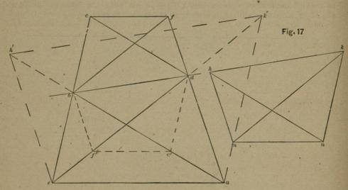
have the sides meeting at b and n cases, according as mn is above or below mutually parallel. Let the bases ae and bk, but we have proved them both. hk be invariable but let the vertex b be Now in Fig. 16 let all the joints in the removed to any point d such that bd || hk, upper chord be removed to v, then the then will the vertex n be removed to a segments  $ea_2$ ,  $a_2a_3$ , etc., are unchanged, point m such that  $mn \parallel ae$ .
