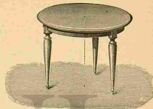
Fig. 13.—Equilibrium of a Body supported on a Horizontal Plane at three or more Points.
