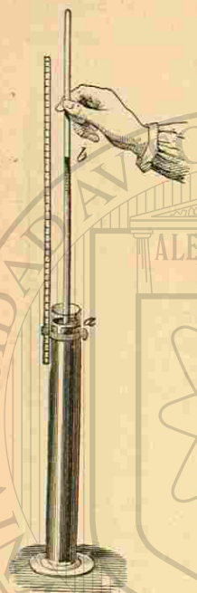
Fig. 121.—Proof of Boyle's Law for Expanding Air.
