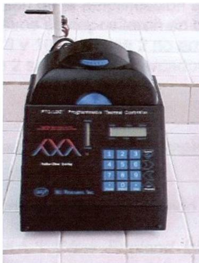
Figura 9. Termociclador PTC-100 ( MJ Research Inc. )
