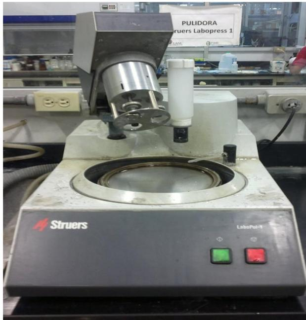
Figura 3.10 Pulidora Struers LaboPOI-1.
