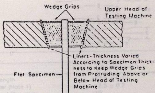
FIG. 2 Wedge Grips with Liners for Flat Specimens
